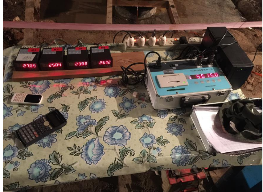
Remote monitoring station using Digital Extensometer (4nos) Load Cell (2nos).
