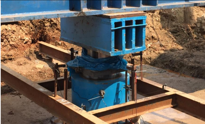
Arrangement of 2x1000T Load Cell for observing load 4 Digital Extensimeter (0.01mm resolution) for observing settlement.
