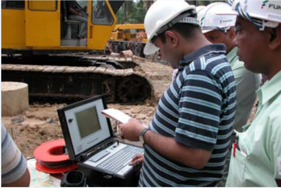
Dynamic Load Testing using Pile Driving Analyzer (PDA) by Pile Dynamics Inc, USA.
