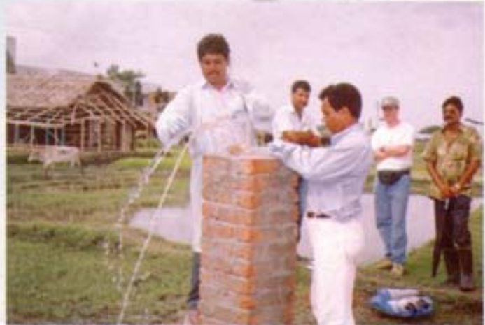
Collection of Water Sample with Teflon Bailor
